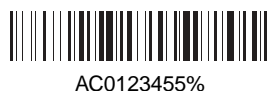
Figure 3. Patient bar code compliant with Health Industry Barcode standard. A signifies the marker for an identifying device affixed to a patient (e.g., a wristband), C is a prefix signifying that the patient identification number follows, 0123455 indicates that the data portion is hospital specific but that a patient identification will be 15 characters or fewer, and the % symbol is the check digit.
