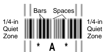
Figure 1. Typical bar code. A = The numeric translation of the bar code (human readable code).
